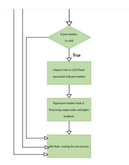
Fig. C1 Programming Flowchart between Processing and Arduino [66]
