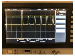
Fig. 8. Oscilloscope of LED panel data in and 5V pins [25]
